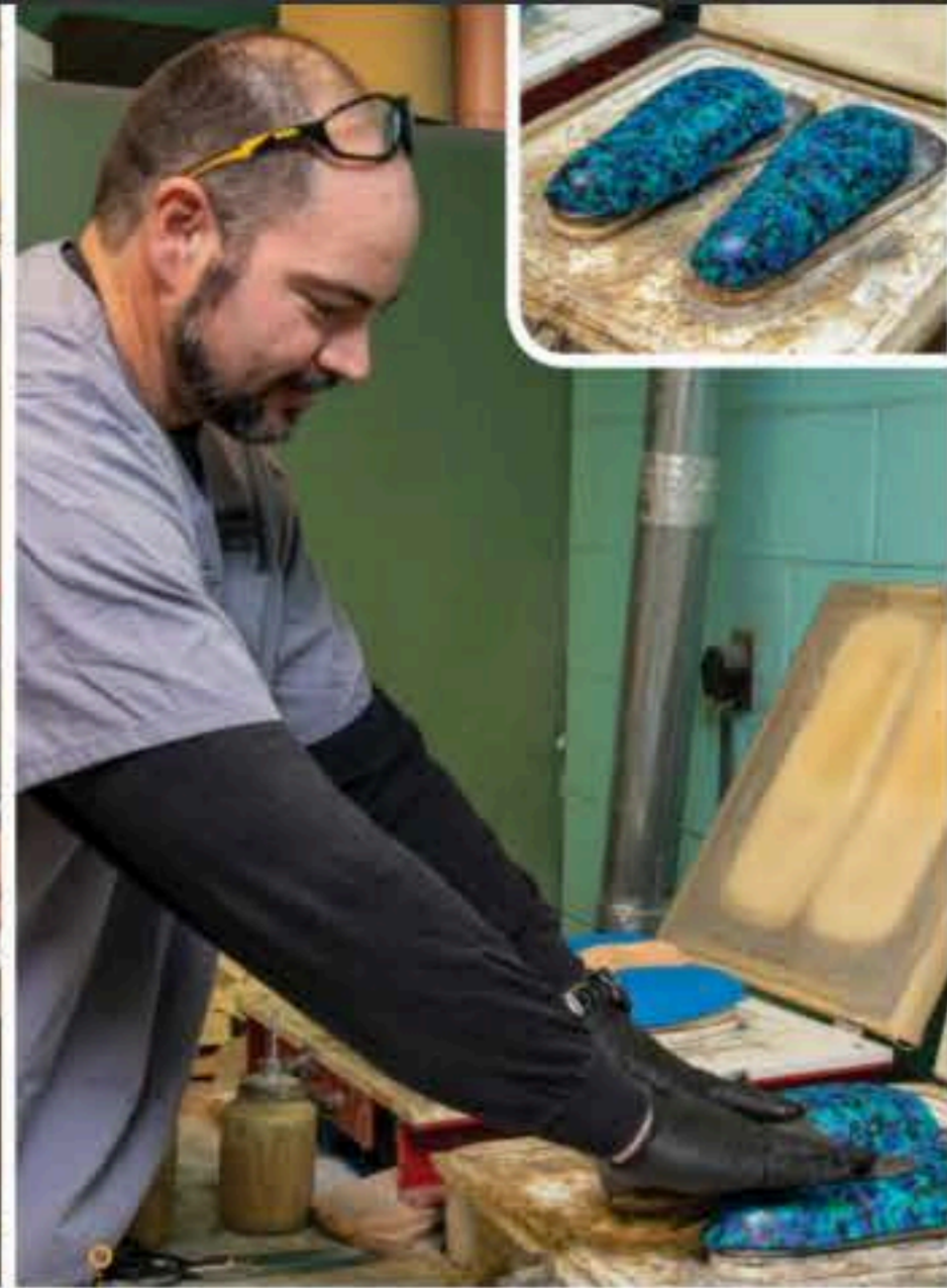
A heat press conforms the material used to develop the orthotic to the foot mold designed specifically for Carly's foot.
