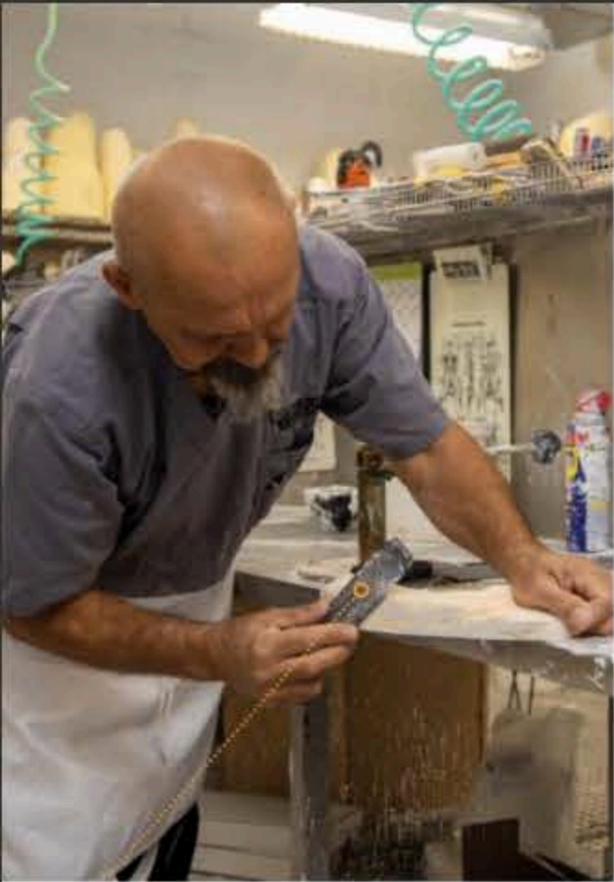
A mold made from an impression of Carly's foot is carefully trimmed of excess material to ensure it will replicate with complete accuracy the orthotic that will be made using it.
